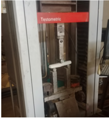
Figure 5: Testometric FS 50 AT testing machine with flexural sample mounted on it.
