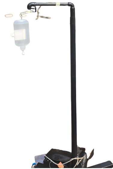
Figure 7: Complete design and construction of the peritoneal dialysis stand.
