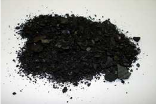
Figure 1: The raw steel mill scale. Source: [10].
