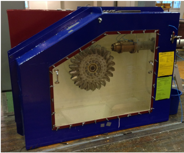
Figure 1: Pelton turbine model used for experimental test in NTNU [10].
