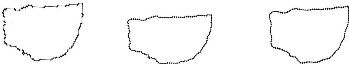
Fig 2.2(a) Original Digitized Outline of Particle Fig 2.2(b) +/- 64 Fourier Descriptors Fig 2.2(c) +/- 24 Fourier Descriptors.
