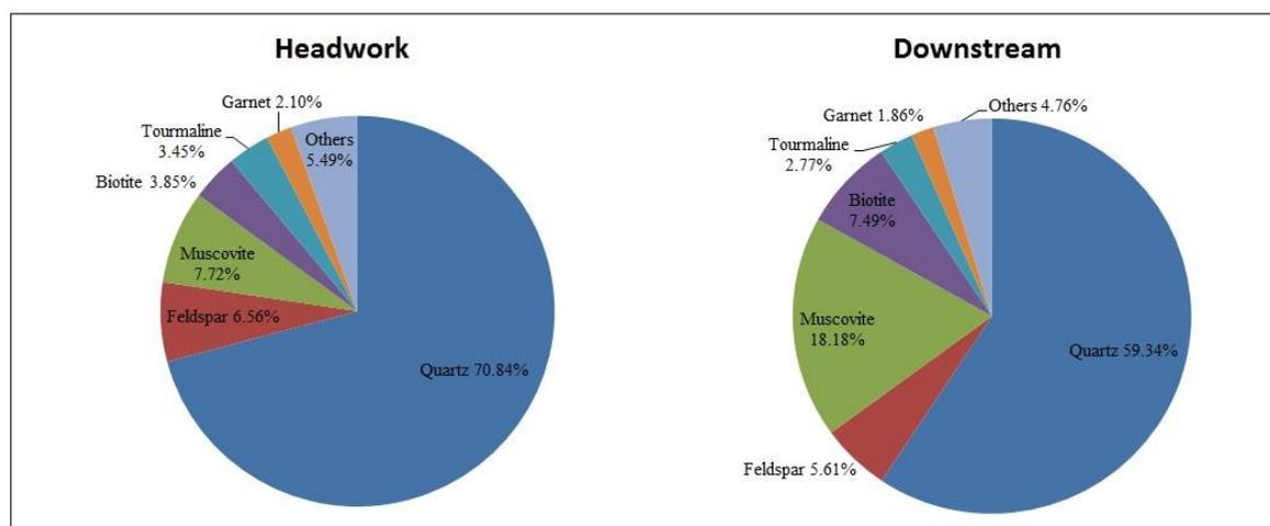
Figure 5 Mineral composition for Jhimruk HPP
