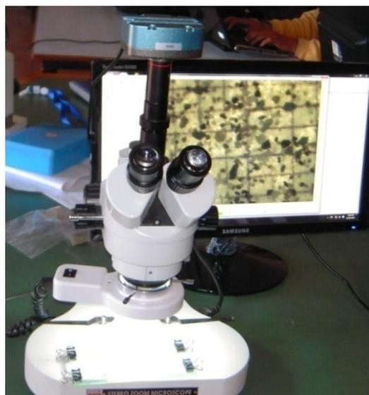
Figure 2 Trinocular Stereo zoom Microscope
