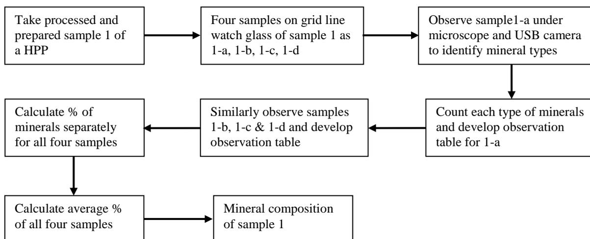
Figure 3 Mineral analysis procedure
