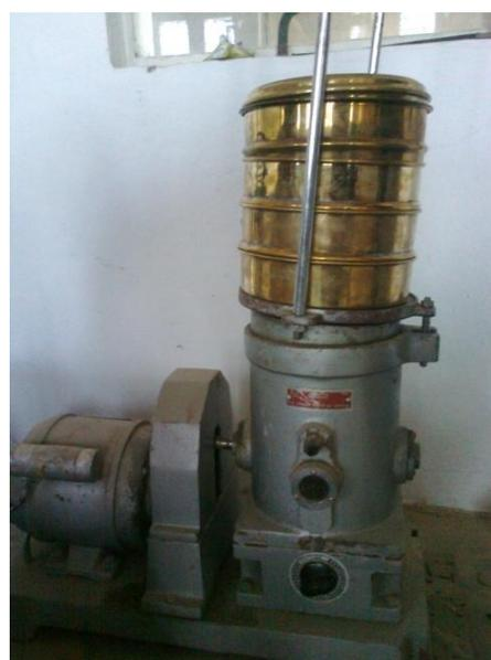
Figure 1 Sieve analysis setup
