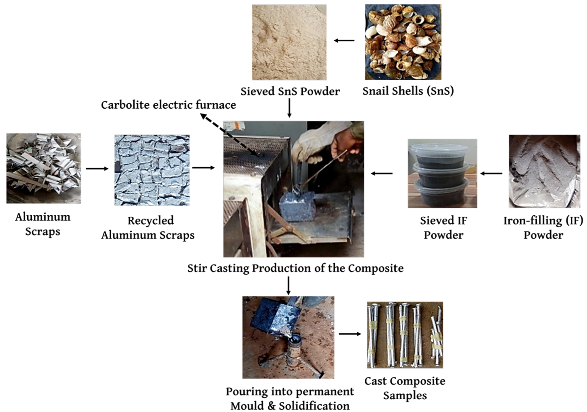
Figure 1: Preparation and production of Al-Fe/SnS hybrid composites
