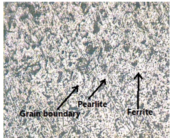
Figure 3: Optical micrograph of the as-received mild steel plate.
