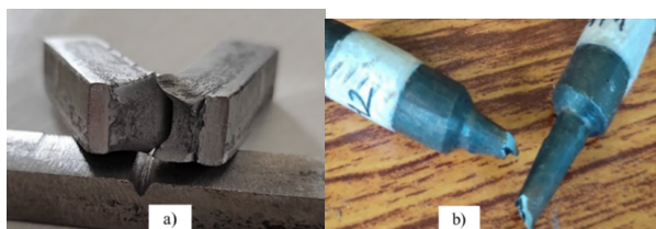
Figure 8: Image of samples after the destructive test. (a) Charpy test sample (b) Tensile test sample.
