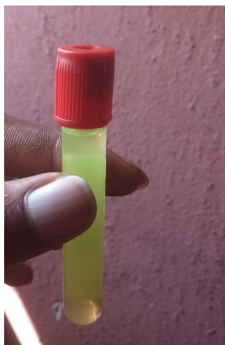
Figure 2: PMS additive from acetone D-limonene and two stroke cycle oil.
